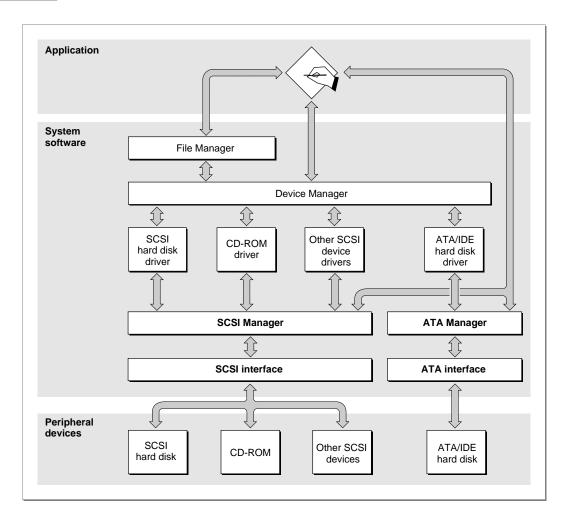
At the system level, the IDE device driver and ATA Manager work in the same way that the SCSI Manager and associated SCSI device drivers work. The IDE hard disk device driver provides drive partition, data management, and error-handling services for the Macintosh Operating System as well as support for determining device capacity and controlling device-specific features. The ATA Manager provides an interface to the IDE hard disk drive for the IDE device driver.
